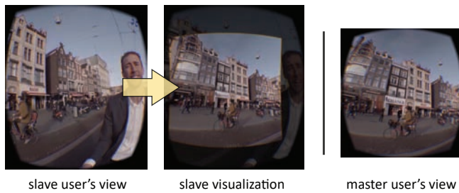
Figure 6: Slave visualization. The master user looks at the bicycle rider (right). The slave user (left) uses “Slaving” to watch the master user’s view. In this mode, the slave’s own view is dimmed and a reduced-size copy of the master full field of view is rendered opaquely on top (middle). This allows the slave user to observe the master’s actions while retaining peripheral self-motion perception. © EU2016NL
