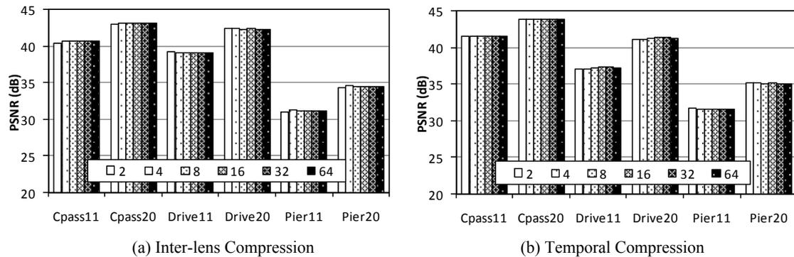
**Figure 8 PSNR Results:** These figures show PSNR results for the Inter-lens (a) and Temporal (b) compression as described in Section 4.2 and 4.3, respectively. Each column represents a maximum vertical search range of 2, 4, 8, 16, 32, and 64.
