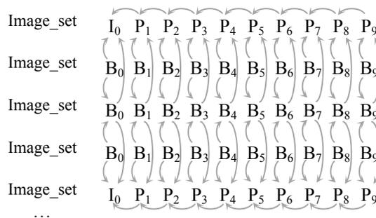
**Figure 2. Typical MVC coding example – This figure shows an example compression of multiview images that is typical in the literature. The image sets (horizontal rows) are images that are taken at the same time.**
