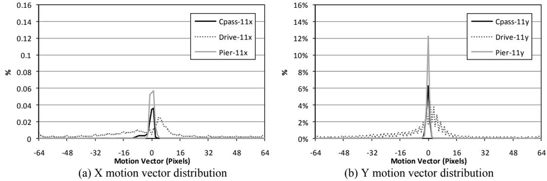
Figure 7 Temporal Predictive-coded Macroblock Distribution: These figures show the X and Y motion vector distributions for macroblocks where at least one of the components was not zero. That is, predictive coded macroblocks with no motion vector are not in the distributions
