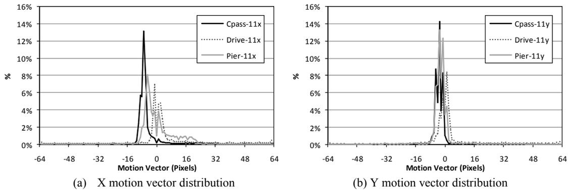
**Figure 6 – Inter-lens Predictive-coded Macroblock Distribution:** These figures show the X and Y motion vector distributions for macroblocks where at least one of the components was not zero. That is, predictive coded macroblocks with no motion vector are not in the distributions
