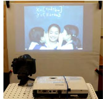
Figure 2. Projector-camera system.
