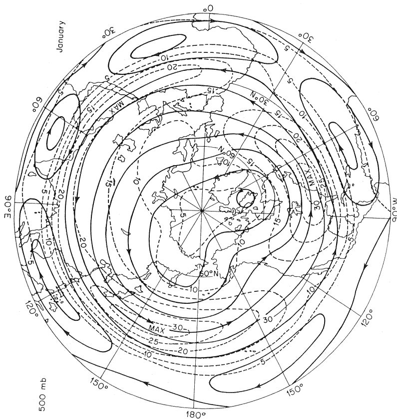
Fig. 8-6 Streamlines and isovels of the Northern Hemisphere mean wind at the 500-mb level in January (speed in meters per second). (From Y. Mintz and G. Dean, The Observed Mean Field of Motion of the Atmosphere , Geophys. Res. Paper, 17, Air Force Cambridge Research Center, Cambridge, Mass., 1952.)
