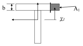
**Problem # S9 :** 2 by 4 Pine wood boards have been glued together to create a composite beam as shown. Assume the dimensions are 2" by 4" (in reality they are less than the nominal value). If the shear strength of the glue is 11 psi, <u>determine the largest load P</u> that the beam can carry w/o glue failure. Assume beam is long enough for the classical beam theory to apply. Do not consider failure due to bending stresses. Answer:90.4 lbs
