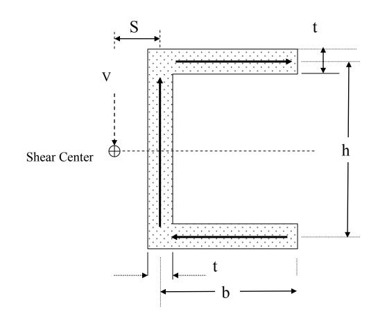
Transverse loads on non-symmetric sections can create twisting torques and warp beam flanges. If such transverse loads are applied at an offset location, the shear forces balance and do not twist the beam. This location is called the Shear Center. For the C-channel shown
