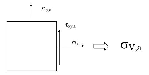
Most common loadings in shafts involves  $\sigma_x$ ,  $\tau_{xy}$ , or both.
