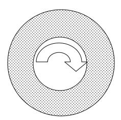
A rotating disk develops substantial inertia-caused stresses at high speeds. The tangential and radial stresses in a disk rotating at  $\omega$  rad/sec is as follows:
