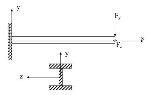
Bending stress for bending about the Z-axis:
