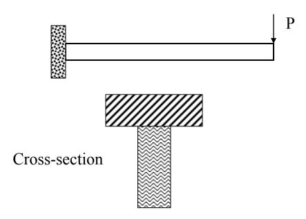
**Problem #S10:** A composite beam is glued as shown. Horizontal members are 1 by 6 inch and the vertical members are  $\frac{1}{4}$  by 10 inch. Transverse load at this cross-section is F=250 lbs. Determine the required minimum glue strength in shear. Answer: 11.8 psi
