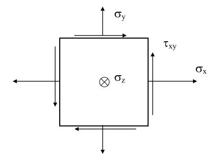
This is a 2D state of stress – only the independent stress components are named. A single stress component  $\sigma_z$  can exist on the z-axis and the state of stress is still called 2D and the following equations apply. To relate failure to this state of stress, three important stress indicators are derived: Principal stress, maximum shear stress, and VonMises stress.
