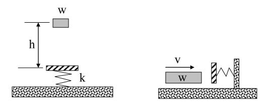
For a falling weight (ignoring the energy loss during impact):
