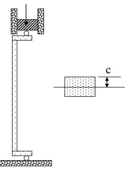
The more general case of column loading is when the load is applied eccentrically. This eccentric load exacerbates the situation as it induces more bending moment due to its eccentricity. The prediction formula is known as the *Secant Formula* which is essentially a classical bending stress formula although it may not look like it. The secant formula is:
