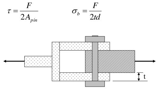
The clevis is also under tear-out shear stress as shown in the following figure (top view):
