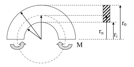
Maximum bending stresses occur at  $r_i$  and  $r_o$  - The magnitude is largest at  $r_i$
