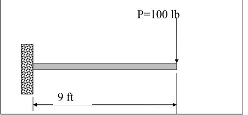
$$\delta = \int_{0}^{L} \frac{M \frac{\partial M}{\partial F}}{EI} dx \quad where \quad M = Px$$
