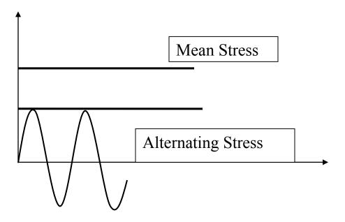
When both mean and fluctuating loads are present, the Goodman criterion is used to determine how much the mean loading affects (reduces) the endurance limit. To begin the analysis, determine the mean and alternating Von Mises stresses. These are actual maximum stresses and they do include the fatigue stress concentration factors. As a result we should be able to calculate the following:
