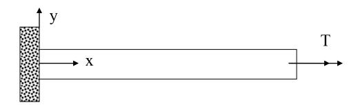
The shear stress is a maximum on the surface of the bar. The state of stress can be represented as a case of pure shear:
