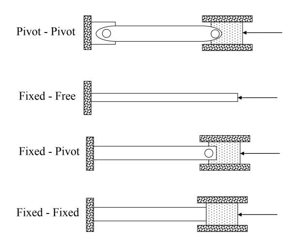
An alternate but common form of the Euler formula uses the "slenderness ratio" which is defined as follows:
