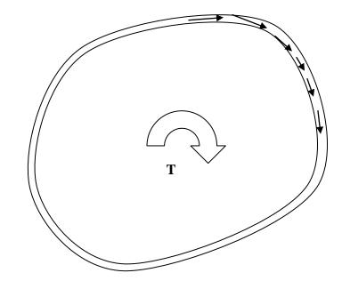
Shear stress in thin-walled tubes (left for closed tubes – right for open tubes)
