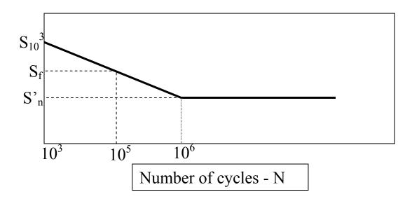
The rotating bending or Moore test endurance limit has to be corrected for the actual part loading and conditions. This includes corrections for surface roughness, gradient effect, and size of the part (in Moore test the specimens are polished, under rotating bending, and are 0.3" in diameter). The result of these corrections is the endurance limit  $S_n$ . Another notation for endurance limit is  $S_e$
