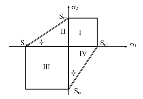
When both  $\sigma_1$  and  $\sigma_2$  are positive (tensile), the fracture is predicted to occur when one of the two principal stresses reaches  $S_{ut}$ . When both  $\sigma_1$  and  $\sigma_2$  are negative (compressive), the fracture occurs when the magnitude of one of the two principal stresses reaches  $S_{uc}$ . The magnitude of  $S_{uc}$  is often more than  $S_{ut}$  as the prior discussion indicated.
