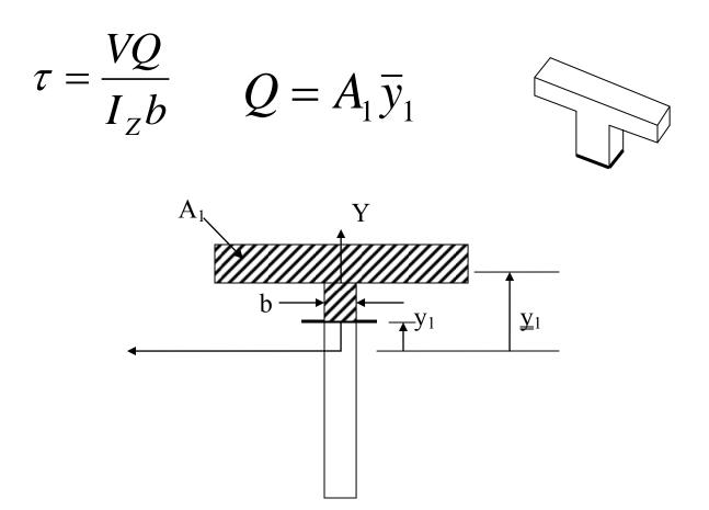
$A_1$  is the area of the cross-section left hanging and  $\underline{y}_1$  is the distance between the centroid of  $A_1$  and the neutral axis (which is the same as the centroidal axis of the entire cross-section).
