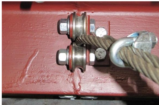
Figure A-8: Upper cable guide as installed on cart
