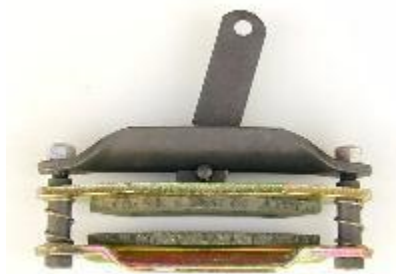
Figure A-1: Transfer case brake caliper as purchased.
