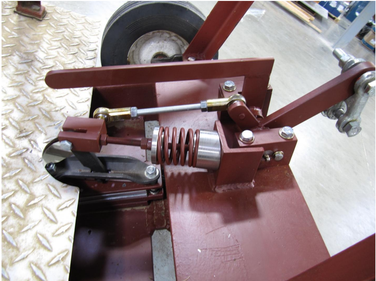
Figure A-13: View of braking system properly installed.
