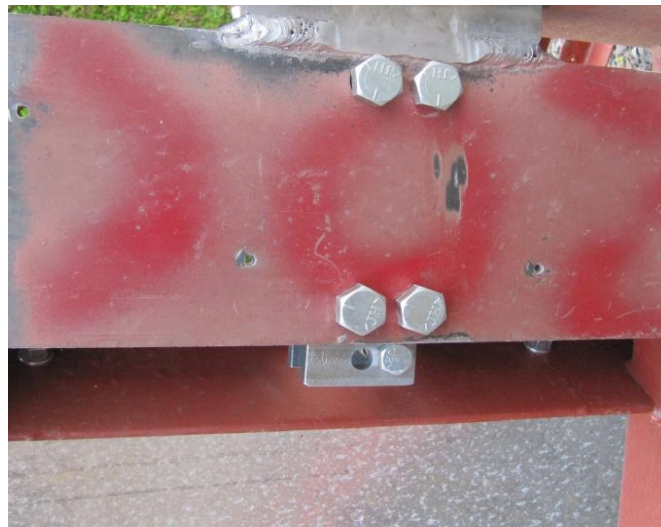
Figure A-3: Brake caliper mounting to the cart as viewed from the bottom.
