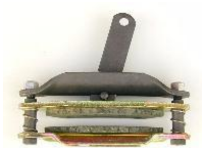
Figure 7: Transfer case brake as purchased.
