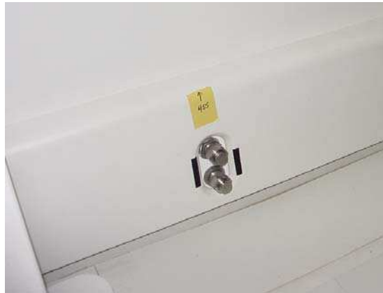
Figure 6A. Multi-User Overboard Vent
