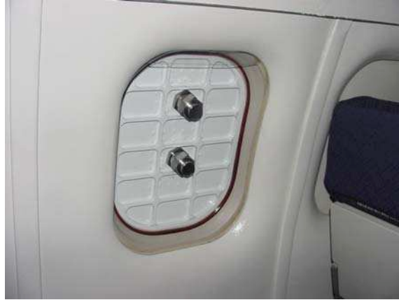
Figure 6B. Dedicated Overboard Vent Ports
