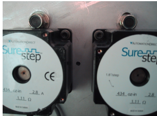
Figure A-1: Mounted stepper motors.
