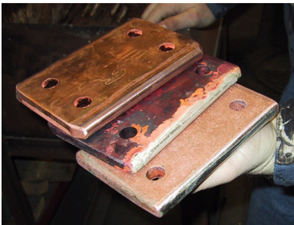
Figure 1: Copper plates at different stages of the brazing process.
