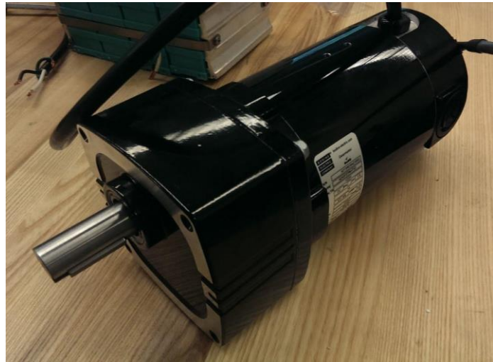
Figure 4 - 42A5-FX Parallel Shaft DC Gearmotor Model 5073
