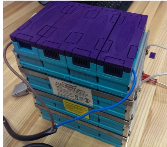
Figure 7 - 12V, 40Ah, LiFePO4 Battery
