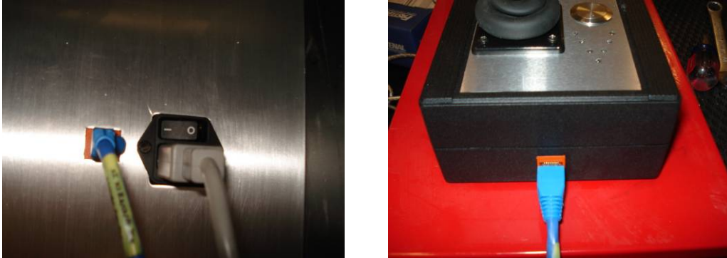
Figure C. 9: Connect a CAT 5 cable to the two orange RJ-45 ports.
