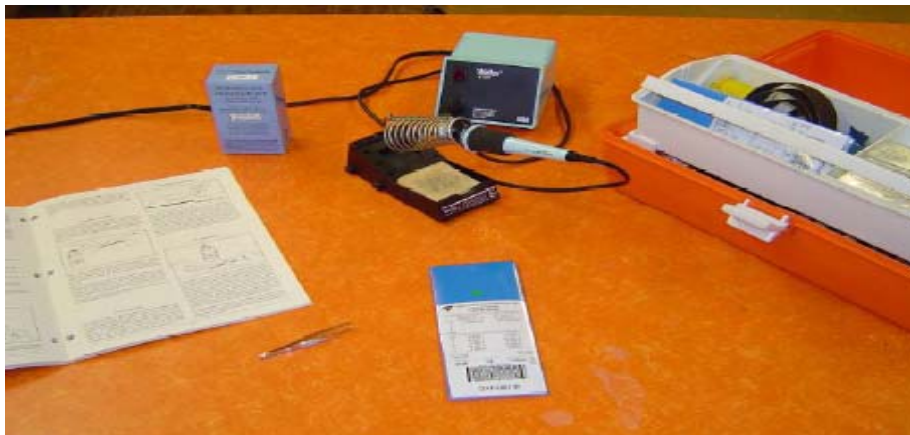
Figure E.A-1: Various supplies to install a strain gage include an installation guide, gages, cleansing chemicals, abrasive sand paper, adhesive, a soldering iron, and related supplies.
