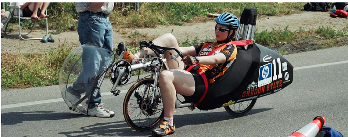
Figure 8.6.6: Example of vehicle with an equivalent strength aluminum roll bar
