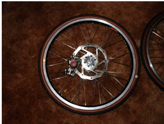
Figure 8.6.18: Disk braking system used in the 2006 PSU HPV
