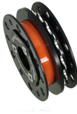
Figure 5.12. Terracycle geared idler selected to improve drivetrain efficiency [Courtesy Robert Johnson]
