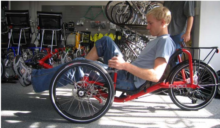
Figure 8.4.11: The Catrike Road uses an adjustable boom.
