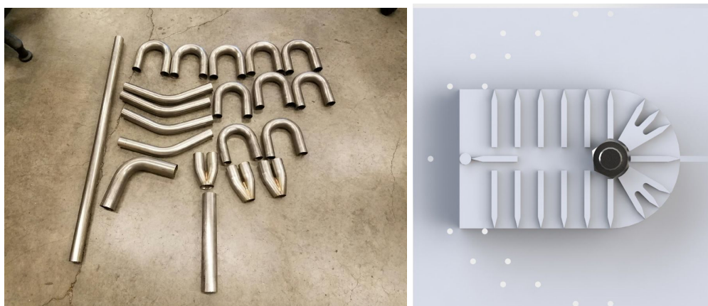
Figure 9. (Left) Raw 304 stainless steel pipes ordered from Columbia River Mandrel Bending . (Right) Cutting jig manufactured from acrylic plastic with adjustable center piece for 45° and 90° cuts
