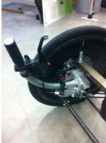
Figure 3. Final steering design for the 2011 HPV, with handlebars connected straight into steering uprights and set and hip level of the rider.
