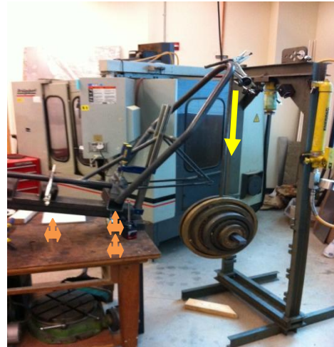
Figure F-3. Boundary conditions of frame RPS testing setup. Orange symbols represent fixture locations. Yellow arrow represents applied load.
