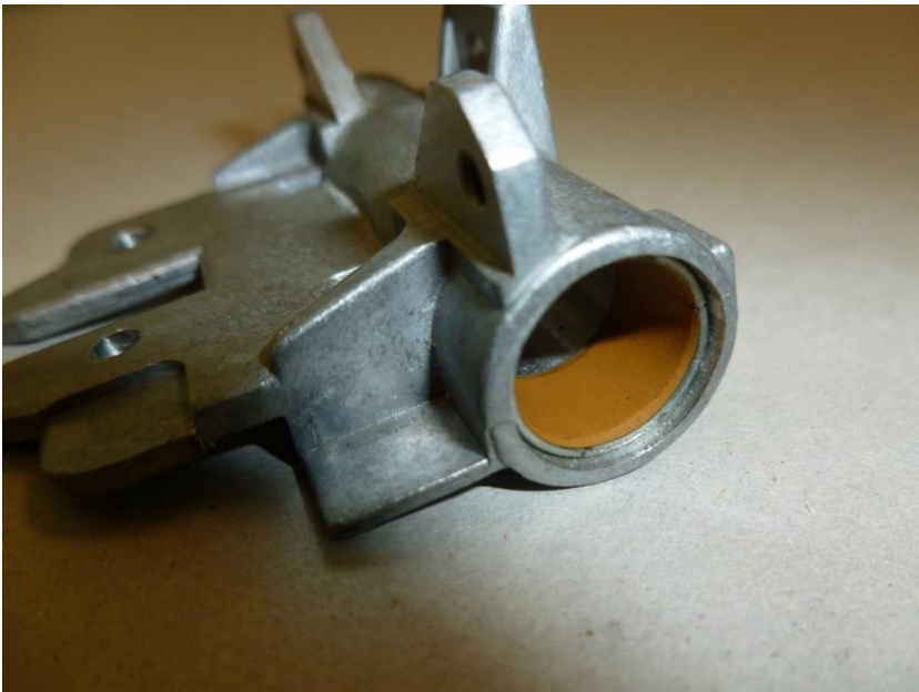
Figure 6-10. Sliding fits often includes two narrow plain bearings at a distance
