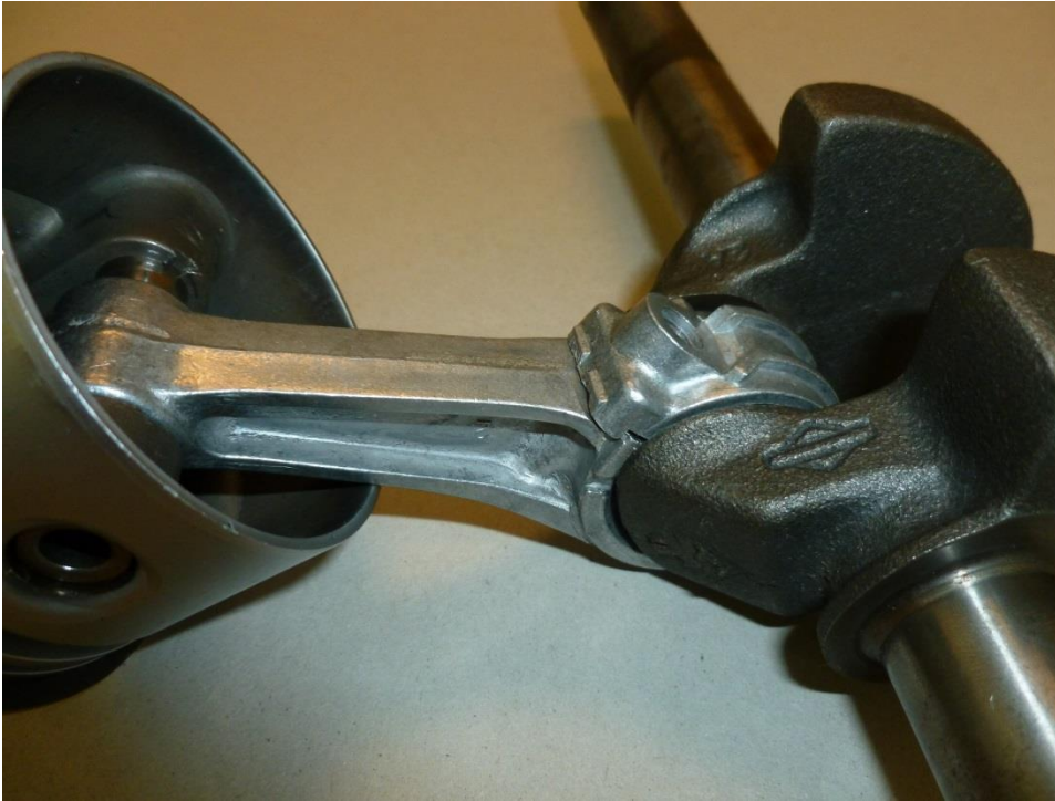
Figure 6-7. Free running fit is adequate for the connecting rod to crank shaft fit
