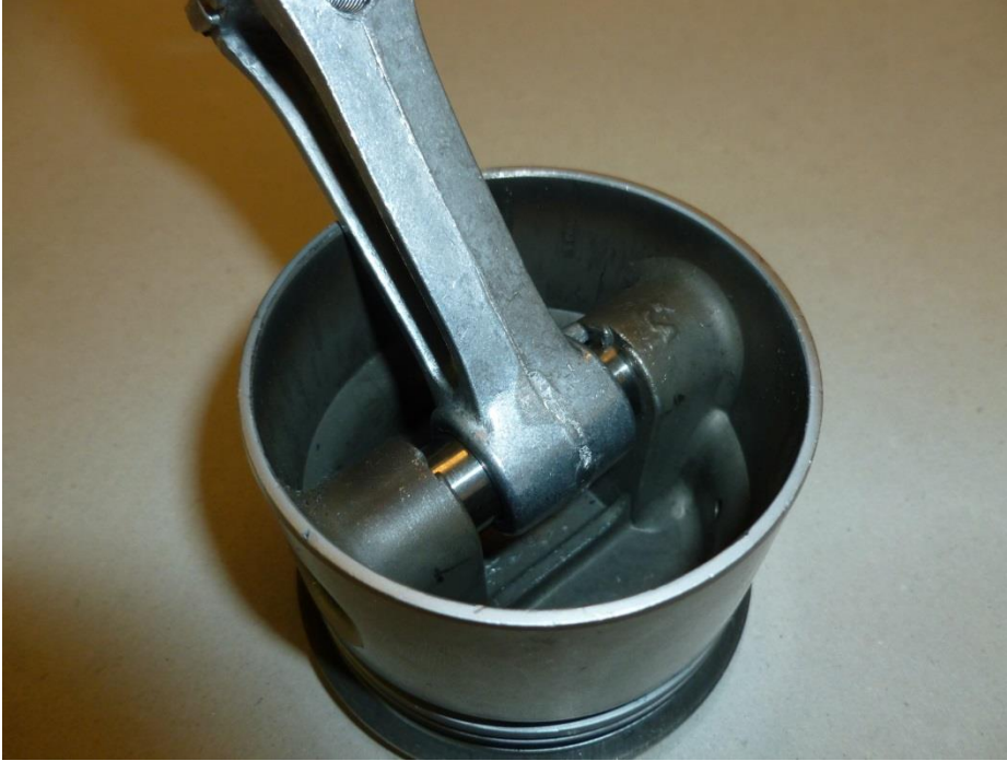
Figure 6-8. Close running fit is adequate for the wrist pin fit to the connecting rod
