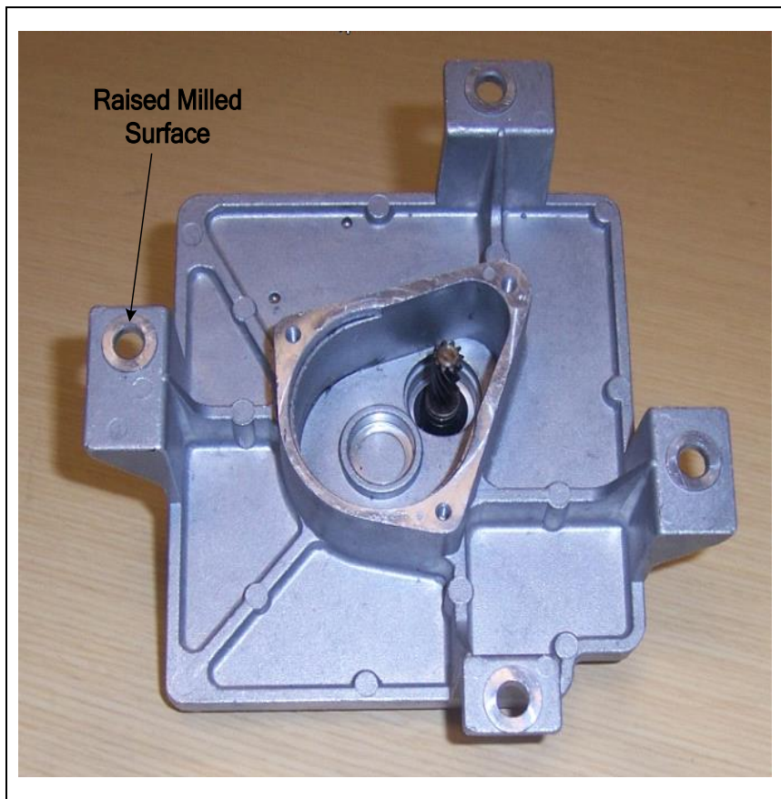
Figure 7-19. Raised and machined surfaces are common in the design of cast parts
