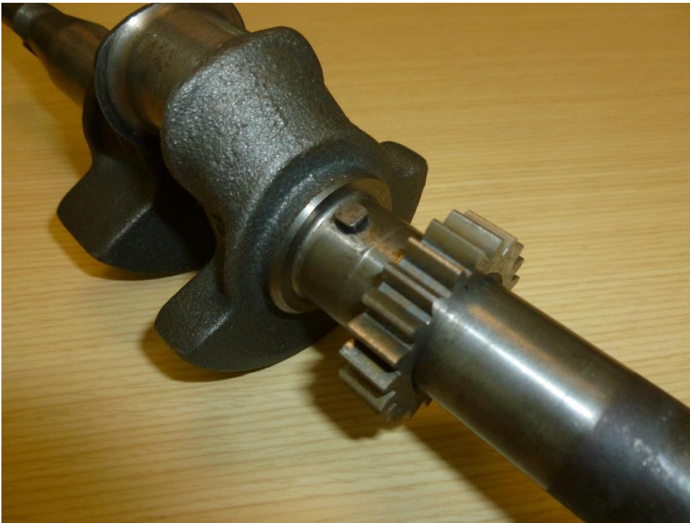
Figure 6-11. Locational clearance fits are adequate for gear fits which often require free assembly with precision centering and little play
