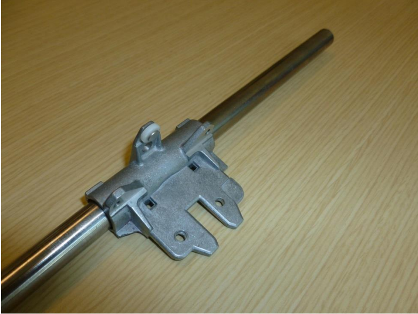
Figure 6-9. Sliding fit is adequate for guide bar fit to the sliding carriage of a printer
