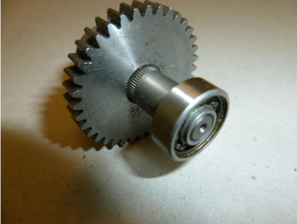
Figure 6-14. Extreme precisions and high forces required for a medium drive fit can be avoided by a serrated shaft surface
