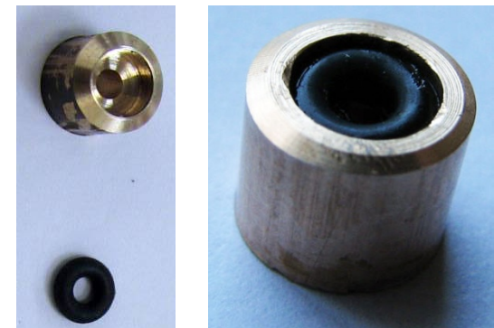
finished bushing / seal
