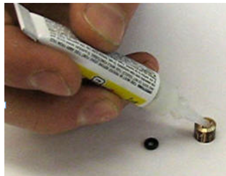
STEP 5: glue in o-ring
