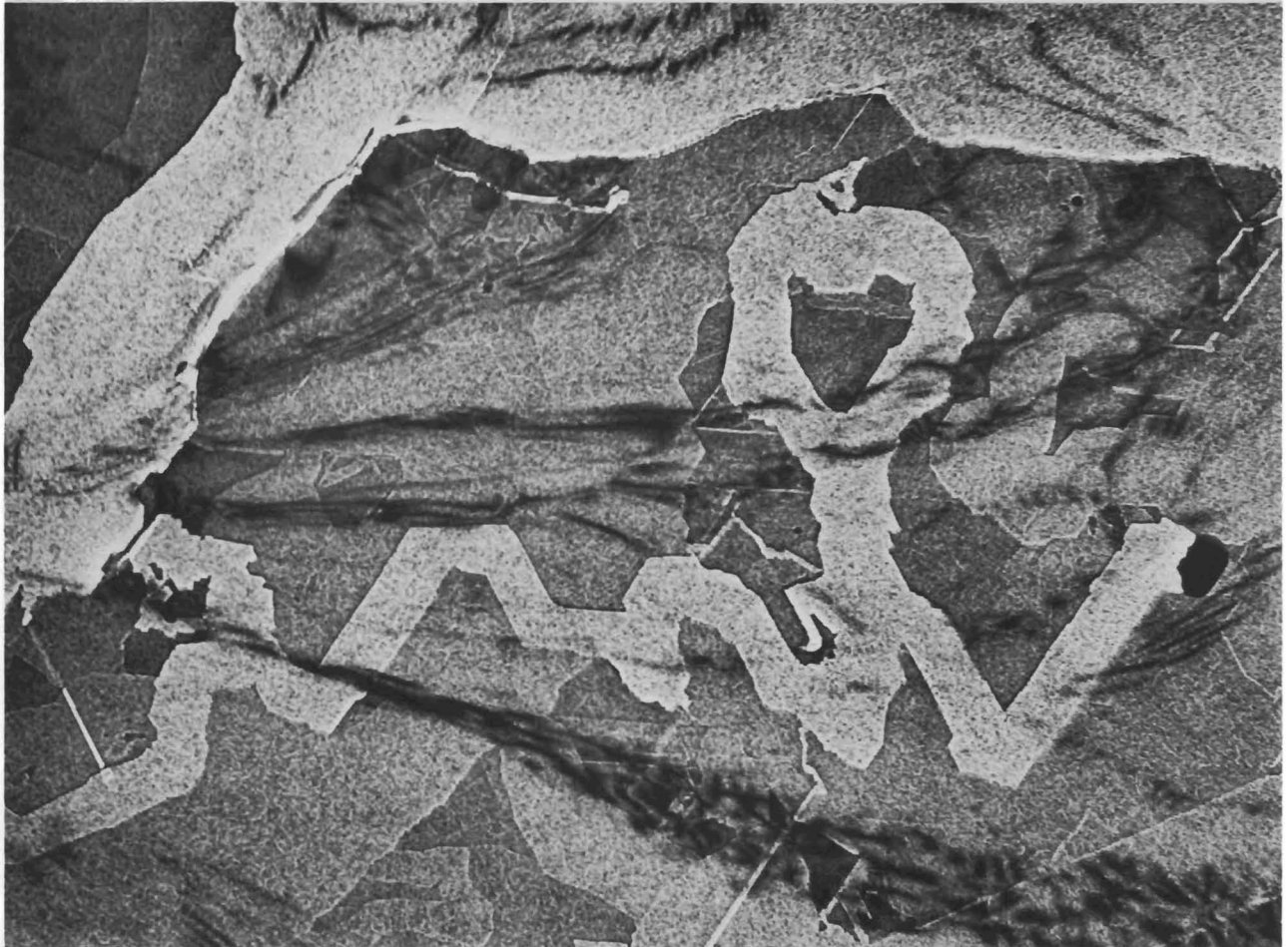
Contrast of reaction channels is enhanced by vacuum deposition of gold. 6,000X 1100°C; P_{\text{H}_2\text{O}} = 4.14 \times 10^{-4} atm. Million Volt Electron Micrograph
