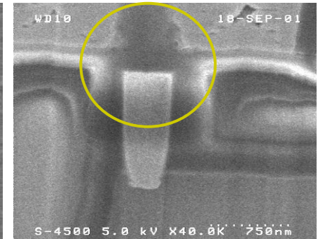
Missing MT6 at Via5
