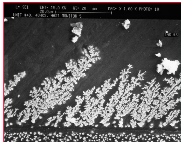
Copper dendrites after 40 hours of biased 156/85 HAST
