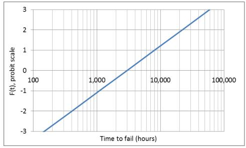
(a) Linear with probit and log time axes means lognormal.
