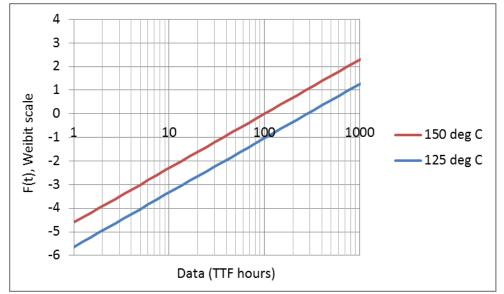
(a) beta = slope =  $\frac{2.3 - (-4.5)}{\ln(1000) - \ln(1)}$  = 0.98 ~ 1. alpha = exp(-intercept/slope) = exp(-(-(-4.5)/0.98) = 97 hr ~ 100 hr.
