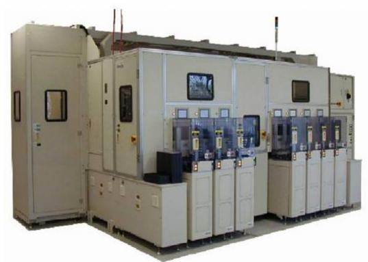
An LCBI burn-in system gives V and T stress to accelerate Si fail mechanisms
