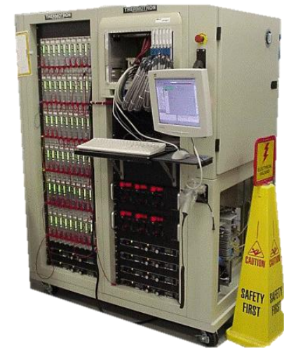
A burn-in system and HAST system perform stress tests on chips
