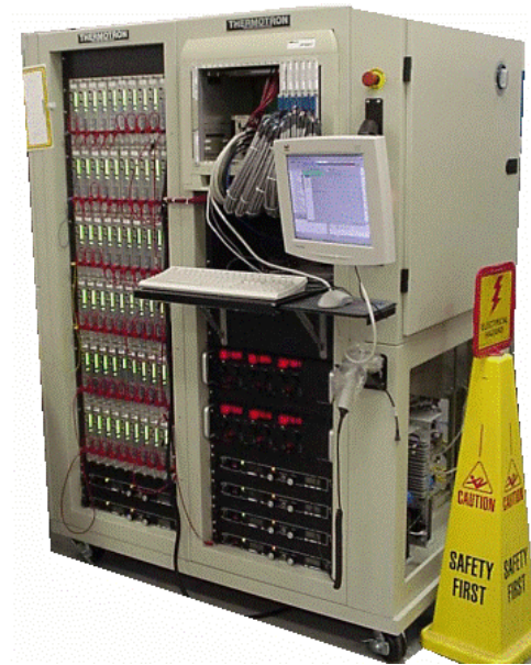
A HAST system gives pressure and humidity along with V and T to accelerate package fail mechanisms
