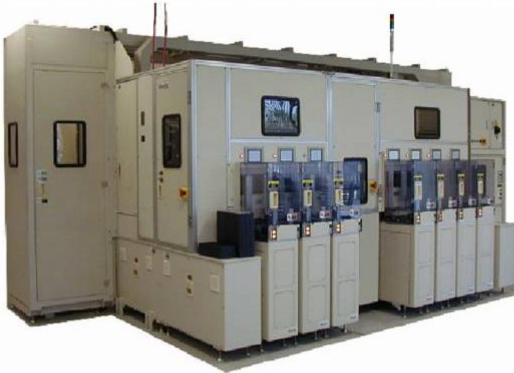
An LCBI burn-in system gives V and T stress to accelerate Si fail mechanisms
