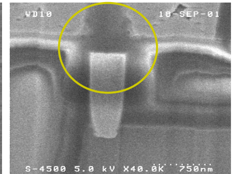
Missing MT6 at Via5
