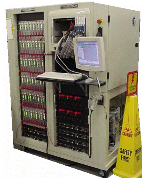
A HAST system gives pressure and humidity along with V and T to accelerate package fail mechanisms
