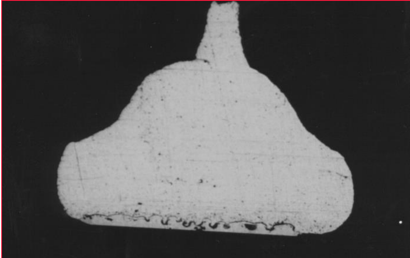
Cross-section of gold ball bond on aluminum pad after 80 hours at 156C/85%RH
