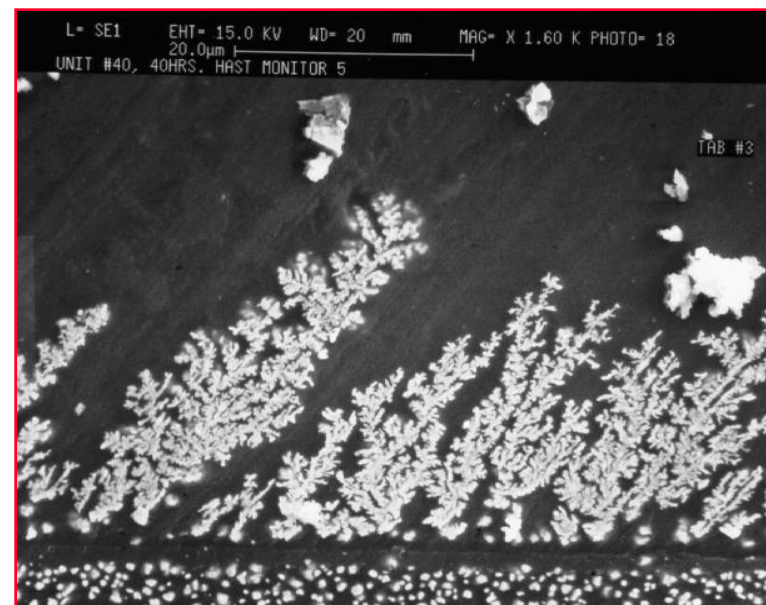
Copper dendrites after 40 hours of biased 156/85 HAST
