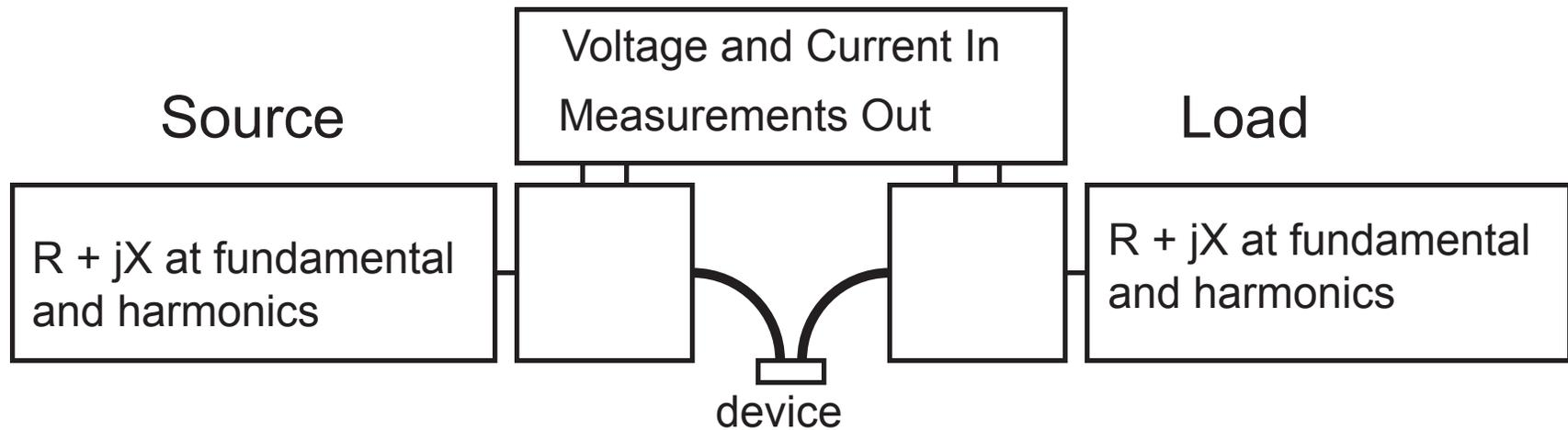
The source and load boxes contain motor driven capacitors that move along transmission lines to present any point on the Smith chart to the Device. Computer control of the motors and data collection, and computer processing of the collected data has made this process much more tedious than in previous decades...oh wait, that wasn't supposed to happen...
