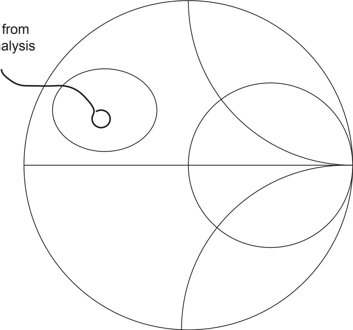
The output of the Load Pull measurements is presented as plots showing optimum load regions under specified conditions
