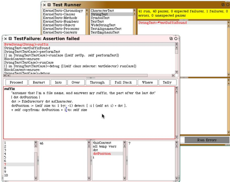
Figure 6.30: Changing the suffix method in the debugger: fixing the off-by-one error after a SUnit assertion failure
