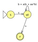
Finally, remove state q0, connecting the start and final state with the regular expression for the self-loop on q0. This regular expression represents all the strings that this NFA accepts.
