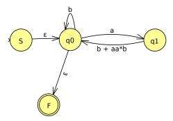
Now remove q1, adding the regular expression for the path through q1 to the self-loop on q0.
