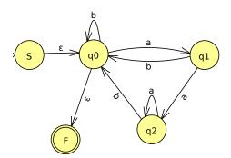
Now we remove state q2, and reconnect state q1 to q0, including the regular expression for the path through q2 along with the original path from q1 to q0.
