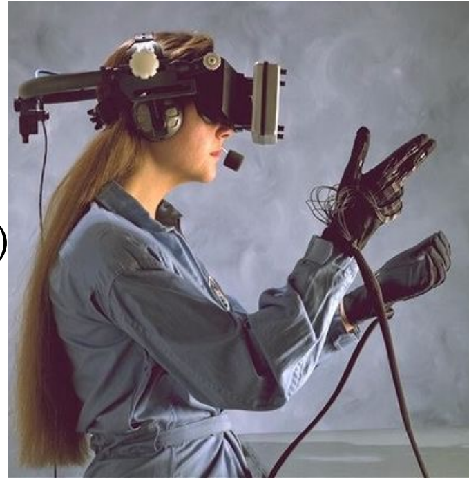
A 1980 HMD and wired gloves at the NASA Ames
