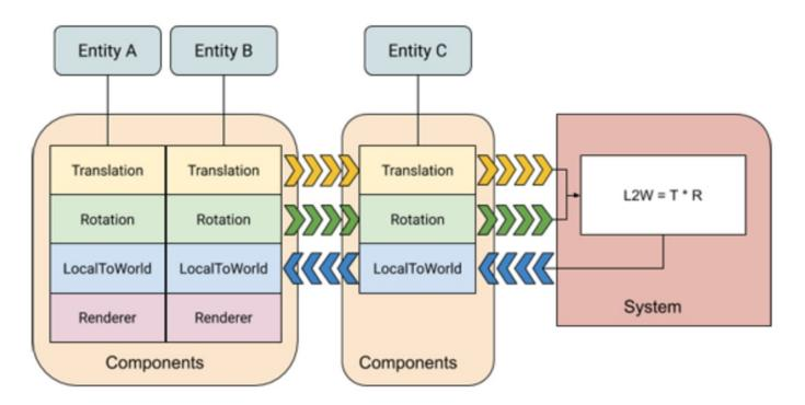
In this diagram, a system reads Translation and Rotation components, multiplies them and then updates the corresponding LocalToWorld components (L2W = T\*R).
