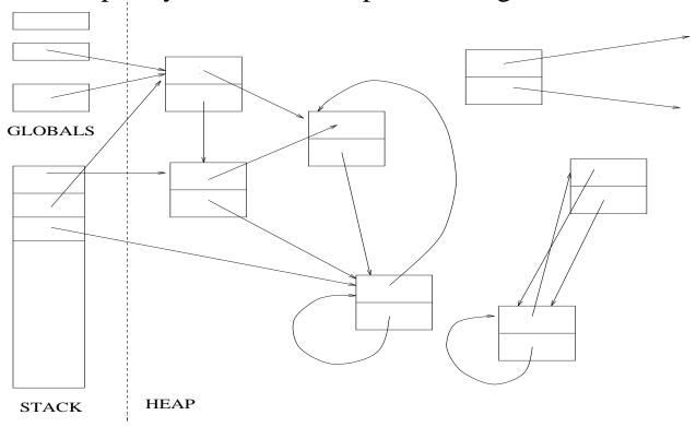
Heap consists of **two-word cells** and each element of a cell is a **pointer** to another cell. (We'll deal with distinguishing pointers from non-pointers later.)
