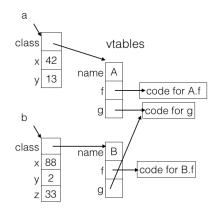
The object records do not change, but the vtables for classes A and B do. Both now have an entry for g pointing to the same code (which A inherits from B. But B now has a different entry in the slot for f than A does. The semantics on slide 14 dictate that the call from b.g() to f should be dynamically dispatched via the vtable slot for b to B.f, rather than being statically resolved to A.f.
