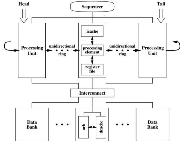
Figure 1: A Possible Microarchitecture of a Multiscalar Processor.
