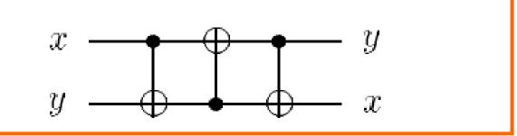
Constructed from three Quantum XORs, we can swap two bits:
