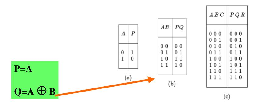
Table GATES: Feynman's truth tables: (a) NOT, (b) CONTROLLED NOT, (c) CONTROLLED CONTROLLED NOT.
