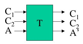
If the two control input bits  $C_1$  and  $C_2$  of a **Toffoli Gate** are both 1, then the input bit A reverses, else all 3 bits go through unchanged.
