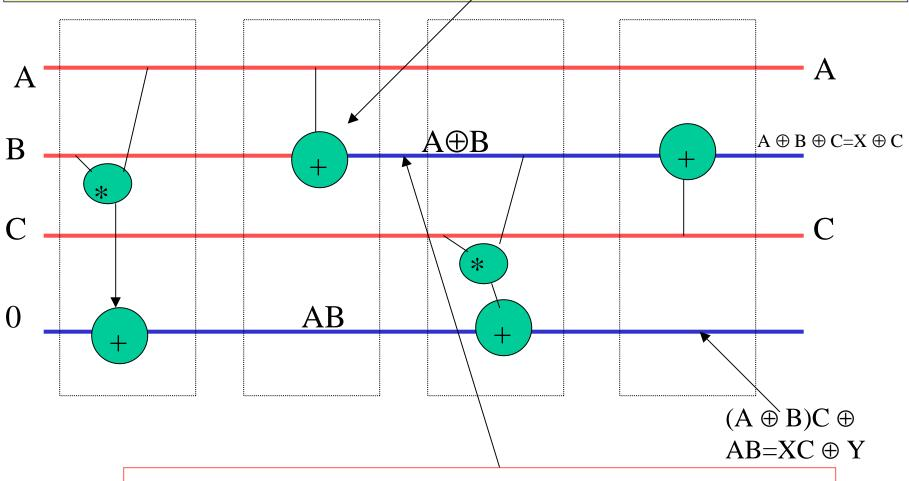
Observe that variable B is no longer useful since output functions can be expressed only in terms of functions  $X=A \oplus B$  and Y=AB
