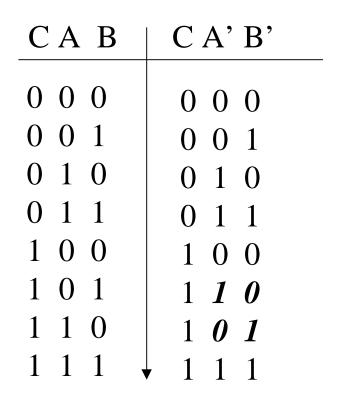
Truth table for the **Fredkin Gate**. If C=1, A and B swap, otherwise A and B go through unchanged.
