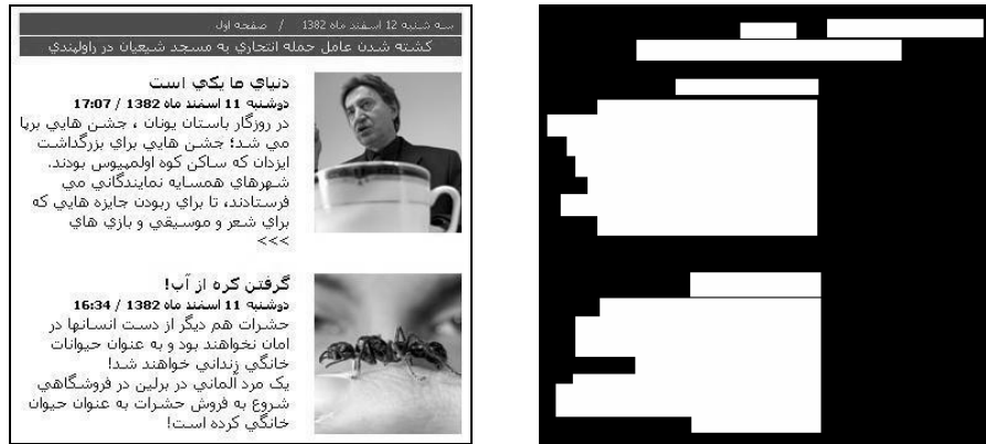
(a) A part of a Farsi document (b) The text mask of (a) Figure 2.1. A document image and its corresponding text mask.
