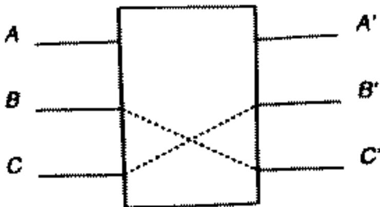
Figure 1: Fredkin gate. The top *control* input goes through unchanged ( $A' = A$ ), and the bottom inputs either go straight through also (if  $A = 1$ ) or cross (if  $A = 0$  then  $B' = C$  and  $C' = B$ ).
