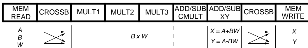
Figure 5.8: Spiffee’s nine-stage datapath pipeline diagram
