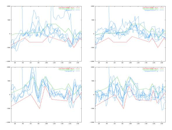
Figure 4: Comparison of original walking gait (left column) and walking gait with motion compensation (right column) in the saggital (top row) and lateral (bottom row) plane.
