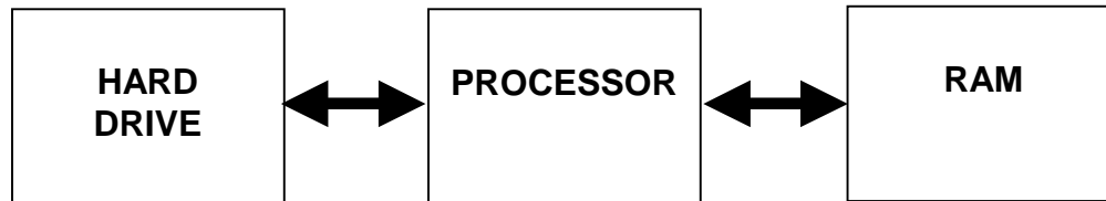
Figure 2.2 Simplified block diagram of main computing components used in a modern PC.
