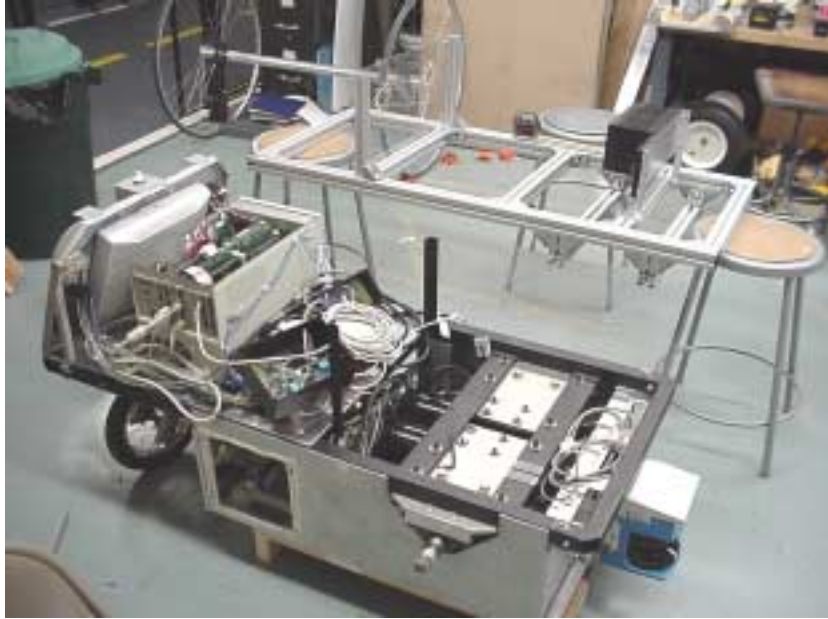
Figure 3.6 Navigator just before installing new aluminum frame.
