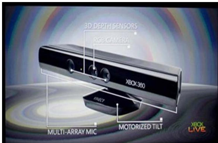
Figure 1: Kinect devices: RGB camera, infrared laser projector, monochrome CMOS camera, multi-array MIC and motorized tilt
