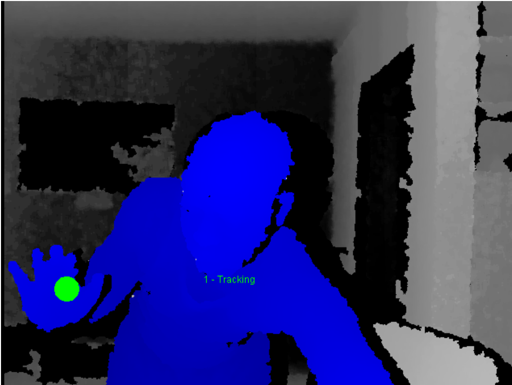
Figure 7 Hand tracking using Joint information
