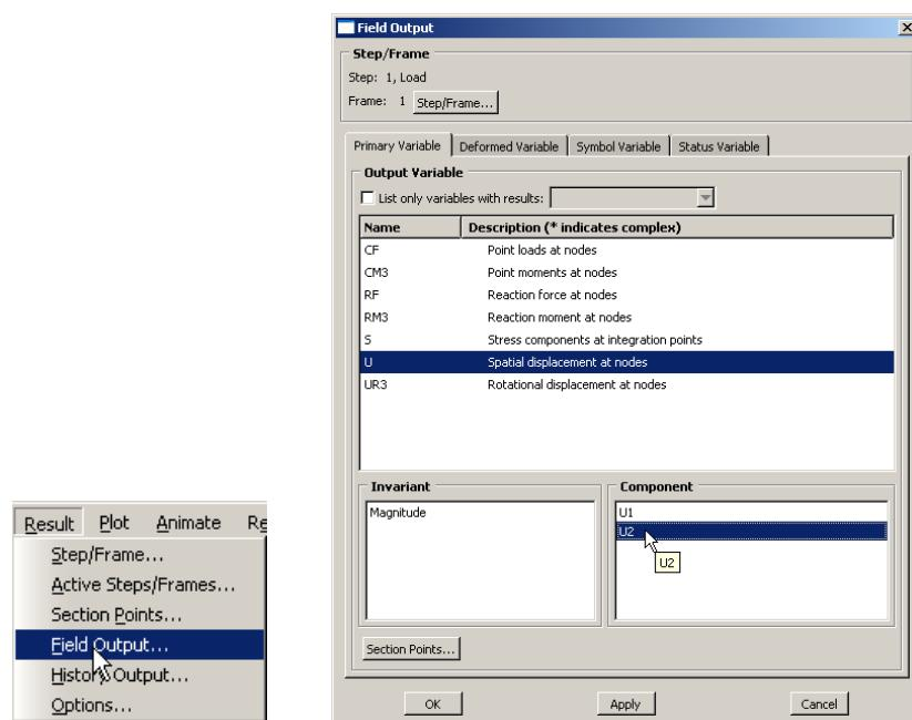
30. To create a text file containing the stresses, vertical displacements, and reaction forces (including the total), in the menu bar click on Report → Field Output
