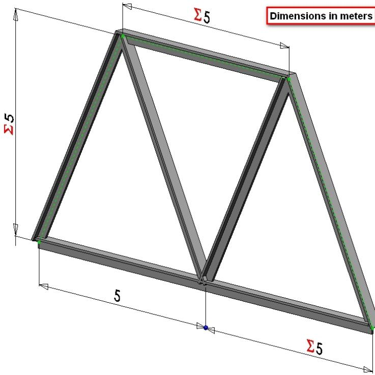
The two dimensional bridge structure, which consists of steel T-sections, is simply supported at its lower corners. A uniform distributed load of 1000 N/m is applied to the lower horizontal members in the vertical downward direction. Determine the stresses and the vertical displacements.
