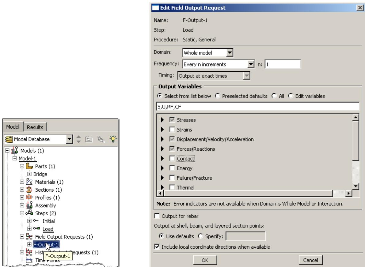
12. Expand the History Output Requests node in the model tree, and then right click on H-Output-1 (H-Output-1 was automatically generated when creating the step) and select Delete
