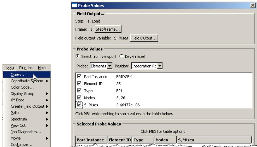
29. To change the output being displayed, in the menu bar click on Results→Field Output
